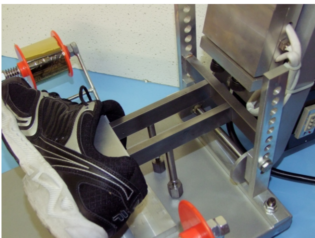
Our optional 'Floating Bed' makes it a possibility to print onto shoes ...
